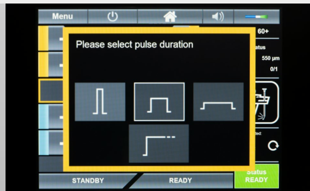
Adjustable pulse lengths and peak power allow for adaptation to the specific properties of the tissue
